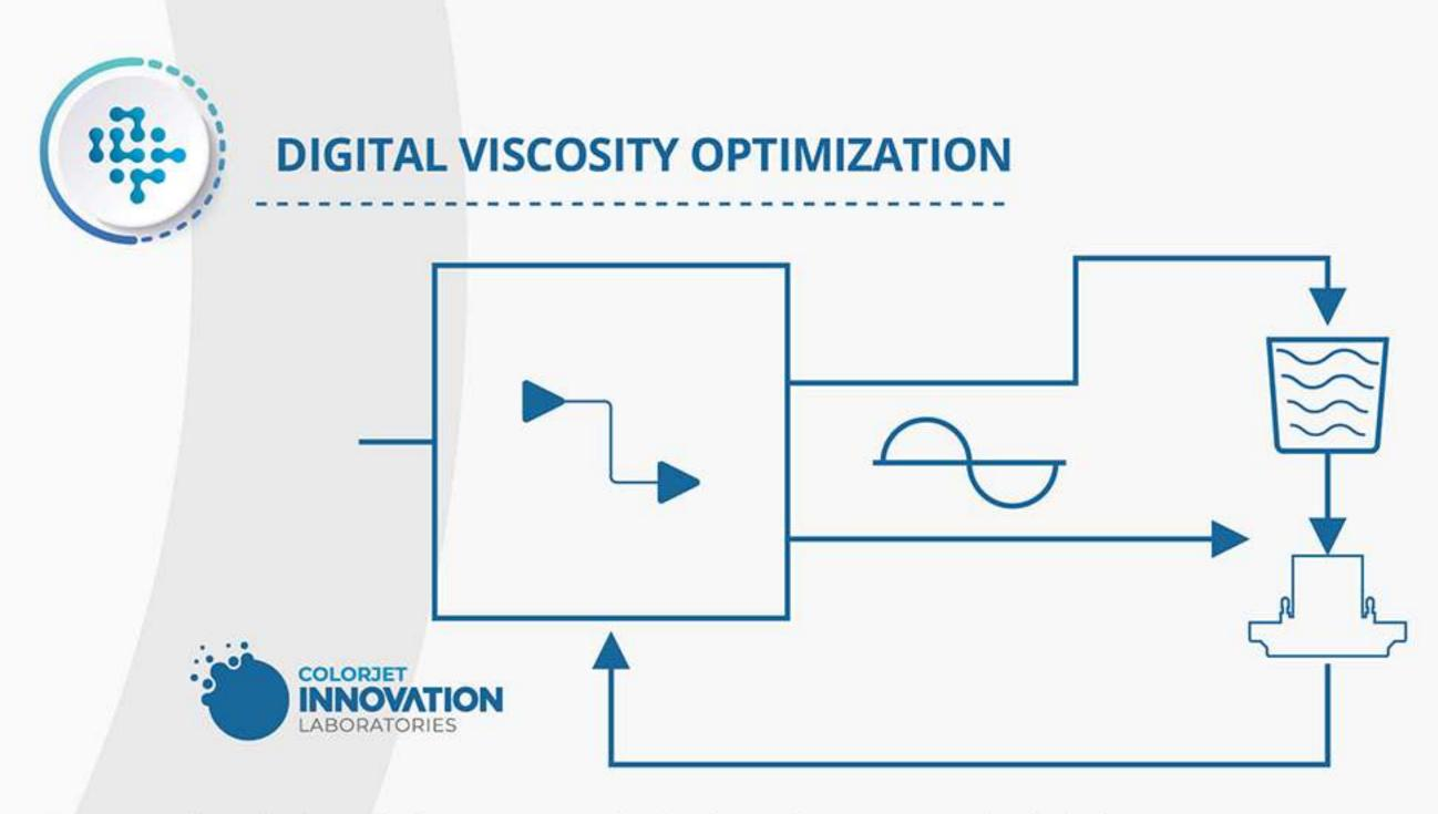
Optimized with digital observation of **Ink viscosity curve**, which helps in maintaining a stable waveform of jetting and ensures constant print quality.
