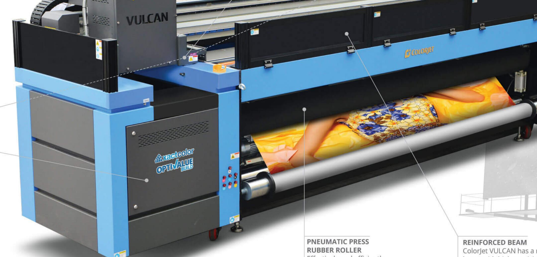
Effectively and efficiently controlling the media tensioning that reduces steps problem and also offer wrinkle free printing.
